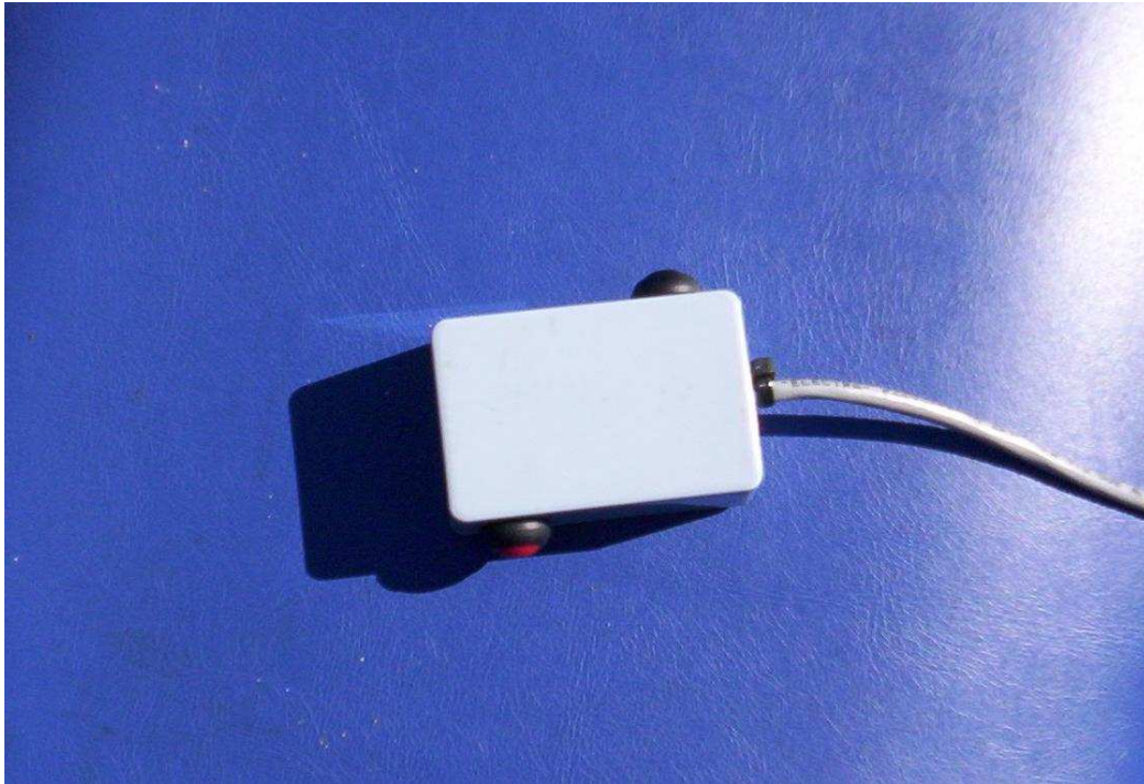
Dead Man's (red) and Dynamic Brake (black) Buttons, resting on the drivers seat.
